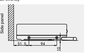
3. Rotate adjustment wheel to achieve suitable door gap
