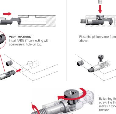
By turning the pinion screw, the threaded dowel makes a synchronized rotation.
