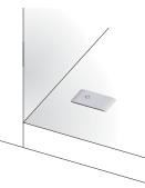
Recommended 2 pan head wood screws  $\emptyset$  3,5 x 16 mm CONNECTINGS
