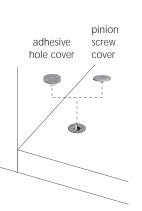
Press strongly with PZ2 cross screwdriver to slot the pinion screw in.
