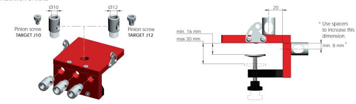
DRILLING SPACERS FOR OTHER PANEL THICKNESSES
