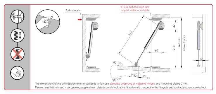
For pistons quantity to be specified according to door size, refer to the chart for "KRABY 244 mm - DROP DOWN".
