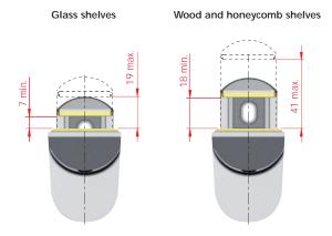
Shelf is clamped between a layer of ridged plastic on both the lower and upper side (coloured parts).
