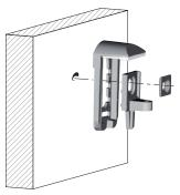
Recommended fixing countersunk screw type - head Ø 5 mm max.
