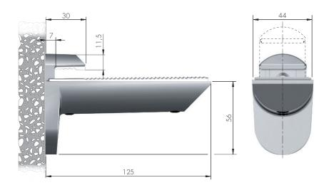
NOTE: KAIMAN is supplied in carton box including 2 pieces, accessories and fitting guide. Countersunk fixing screws  $\varnothing$  5x50 and rawlplugs Fischer SX  $\varnothing$  8x40 to wall are included.
