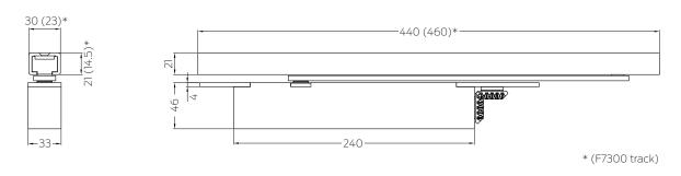
(Dimensions for F7300 track)\* All measurements are in mm.
