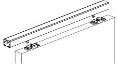
(b) Locate the hanger bolt into the bracket opening until the locking lever clips into the locked position.
