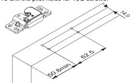
(c) Fix bracket with mounting screws provided.
