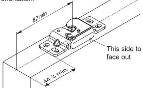
(b) Pre-drill the pilot holes for 10G screws.
